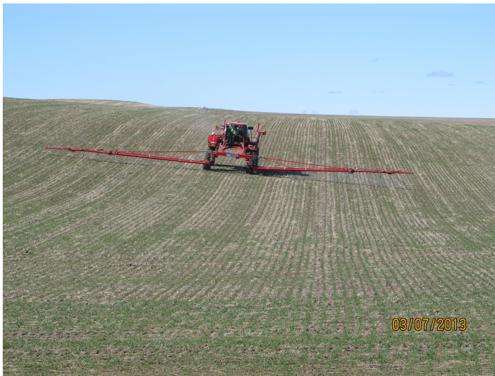
Figure 9. Jepsen's sprayer has auto-steer, auto boom section control, and auto rate control. Photo: Bill Jepsen.
