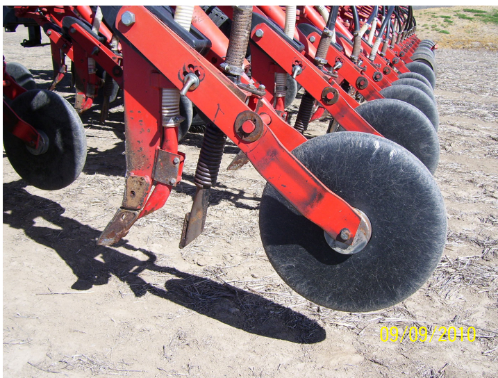
Figure 6. A close-up showing the openers on Jepsen’s Coserva Pak Drill. Photo: Bill Jepsen.
