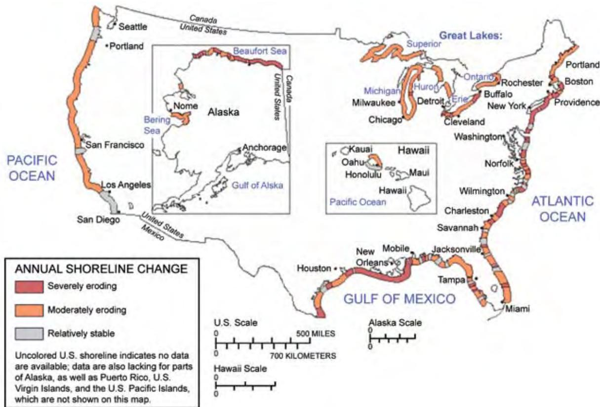
**Figure 1.8** Shoreline change around the United States based on surveys over the past century. All 30 coastal states are experiencing overall erosion at highly variable rates due to natural processes (e.g., storms, sea-level rise) and human activity (From USGS, 1985).
