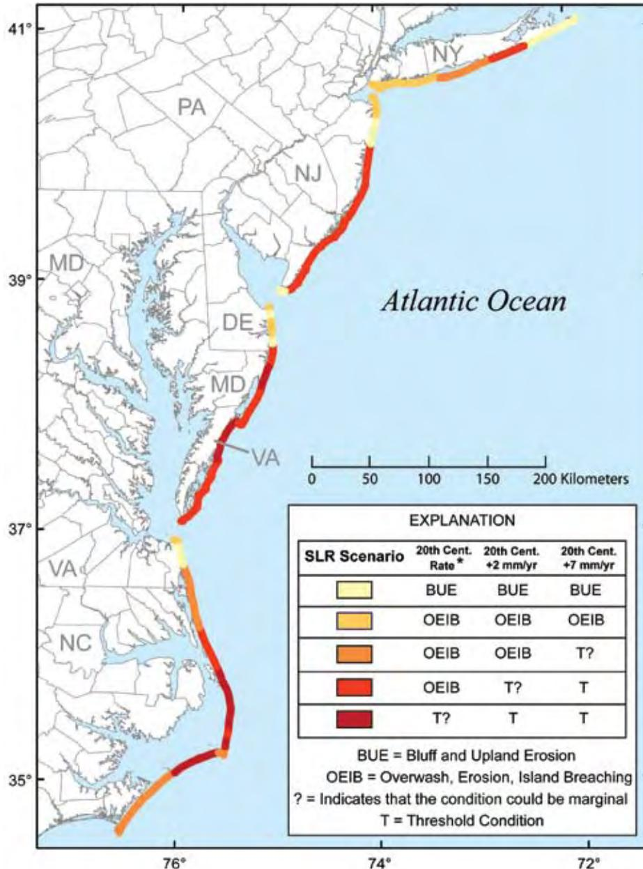
**Figure 3.2** Map showing the potential sea-level rise responses (in millimeters [mm] per year [yr]) for each coastal compartment. Colored portions of the coastline indicate the potential response for a given sea-level rise scenario according to the inset table. The color scheme was created using ColorBrewer by Cindy Brewer and Mark Harrower. After Gutierrez et al. (2007).
