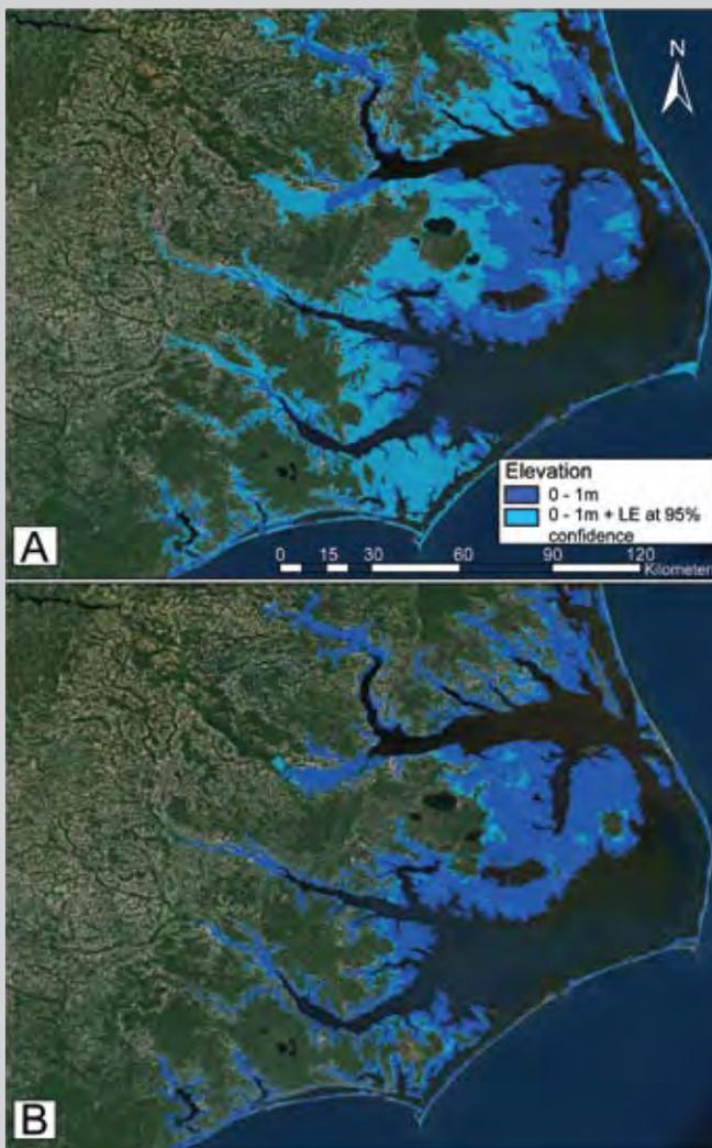
**Box Figure 2.1** (A) Lands vulnerable to a 1-meter sea-level rise, developed from topographic map-derived DEMs and (B) lidar elevation data (Gesch, 2009). The background is a recent true color orthoimage.
