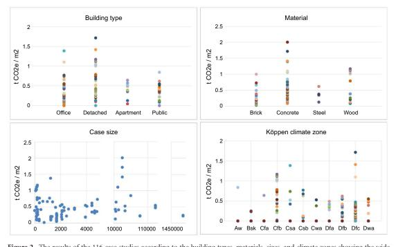
Figure 2. The results of the 116 case studies according to the building types, materials, sizes, and climate zones showing the wide variation even within similar classes of buildings.
