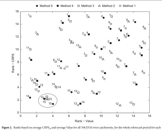
**Figure 2.** Ranks based on average  $CRPS_m$  and average Value for all 768 EFAS river catchments, for the whole reforecast period for each multi-forcing configuration. The numbers indicate the forecast combination (table 1) and the shapes indicate the method used to optimize. The full multi-forcing ensemble is ringed.
