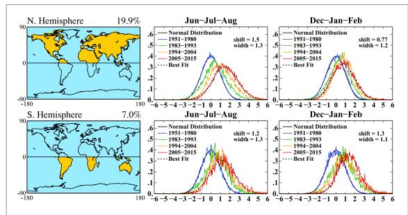
**Figure 1.** Frequency of occurrence of local temperature anomalies (relative to 1951–1980 mean) divided by local standard deviation (horizontal axis) for land areas shown on map. Area under each curve is unity. Numbers above the maps are percent of the globe covered by the selected region. 'Shift' and 'width' refer to the dashed curve fit to 2005–2015 data and are relative to the 1951–1980 base period (see text).
