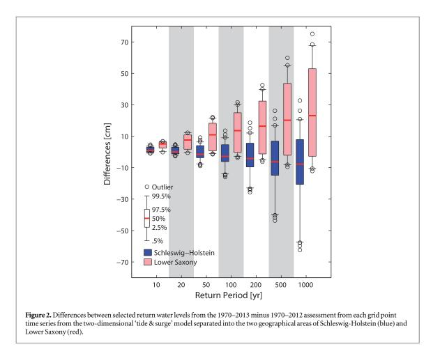
sample starting 1970 and ending from 1999 up to 2013 (small inset in figure 1). In agreement with Arns *et al* (2013), the 200 year return water levels remained stable from 1999 to 2012, but an unprecedented increase is detected when including 2013. This underpins the exceptional influence of storm 'Xaver' on the return water levels along the southwestern coastline of the German Bight.
