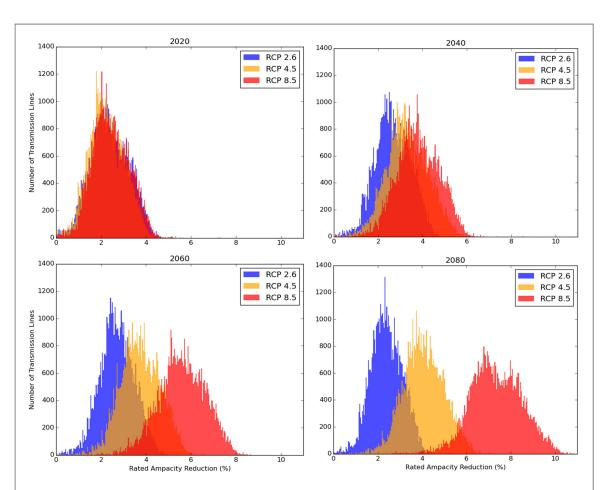
**Figure 2.** Histograms indicating percent reduction to transmission capacity by decade (from top left to bottom right: 2020, 2040, 2060, 2080). RCP scenarios (2.6, 4.5 and 8.5) are indicated by their respective colors (blue, yellow and red). The horizontal axis represents bins of percent ampacity reductions, while the vertical axis represents the number of transmission lines falling into each bin.
