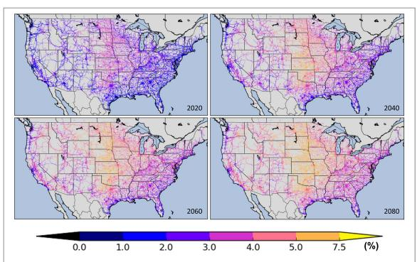
**Figure 1.** Climate attributable reductions to transmission capacity by decade (from top left to bottom right: 2020, 2040, 2060, 2080). Colors indicate the percent reduction in transmission capacity under the average RCP 4.5 scenario, relative to the 1990–2010 reference period. For additional information on transmission line visualizations, see SI section 4.6.
