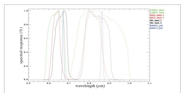
**Figure 2.** Response functions of satellite sensor systems used for calculation of the NDVI BRDF models. Note: AVHRR—Advanced Very High Resolution Radiometer, SPOT—Satellite Pour l'Observation de la Terre, TM5—Landsat Thematic Mapper 5, EnMAP—Environmental Mapping and Analysis Program.
