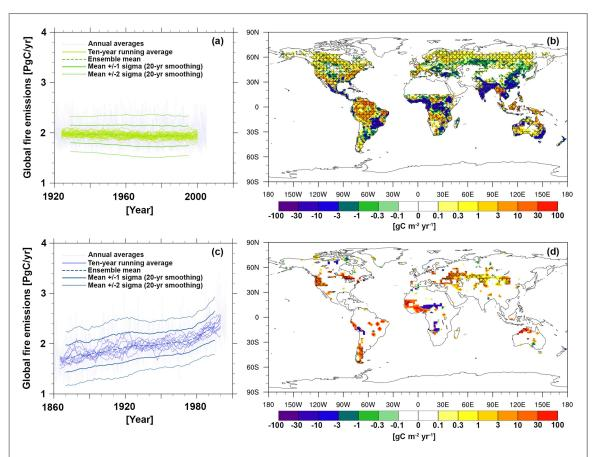
**Figure 4.** Change in annual fire emissions shown as a timeseries of global means for (a) CESM1 and (c) ESM2Mb, and plotted spatially as the difference in mean fire emissions between 1991–2005 and 1920–1934. Hatching indicates grid points for which the difference in means is significant with 95% confidence.
