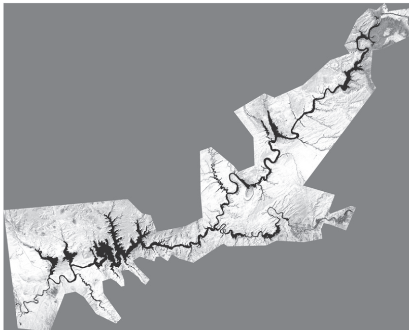
Figure 1. Water mask (black color) calculated with Landsat 5 images (9 June, 2004) over the Lake Powell in USA derived from the approach based on the NDWI and MNDWI index.
