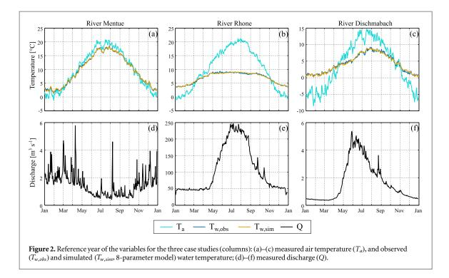
Air and water temperature series should be long enough to capture interannual variability, thus in general should extend for several years. As a general rule, we used 2/3 of the available series for calibration and 1/3 for validation of the model.
