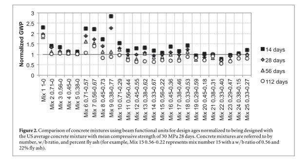
with the production of cement, with the GWP from cement ranging between 5 and 35 times higher than GWP from transportation. This was to be expected because the water content was held nearly constant for all mixtures examined as were, for the most part, the aggregate contents. By holding these constituents constant, the variability in binder content resulted in being the main driver for change in GWP.
