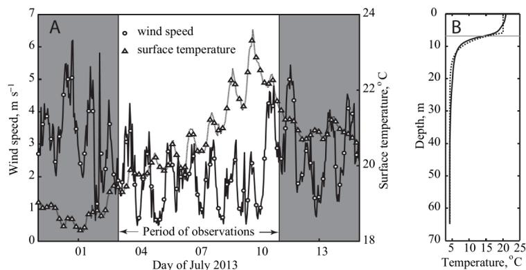
**Fig 2.** (A) Lake surface temperature and wind speed before, during and after the field experiment. (B) The vertical temperature profile averaged over the observations period. Horizontal dash line marks the bottom of the epilimnion determined from location of the maximum vertical temperature gradient.
