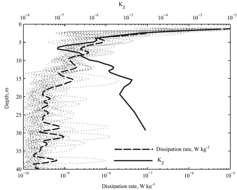
**Fig 3. Turbulent mixing within the water column during the field experiment.** Turbulent diffusion coefficient  $K_z$  averaged for the study period (thick solid line) and the dissipation rate of the turbulent kinetic energy (thin dash lines are individual profiles; thick dash line is the average for the whole study).
