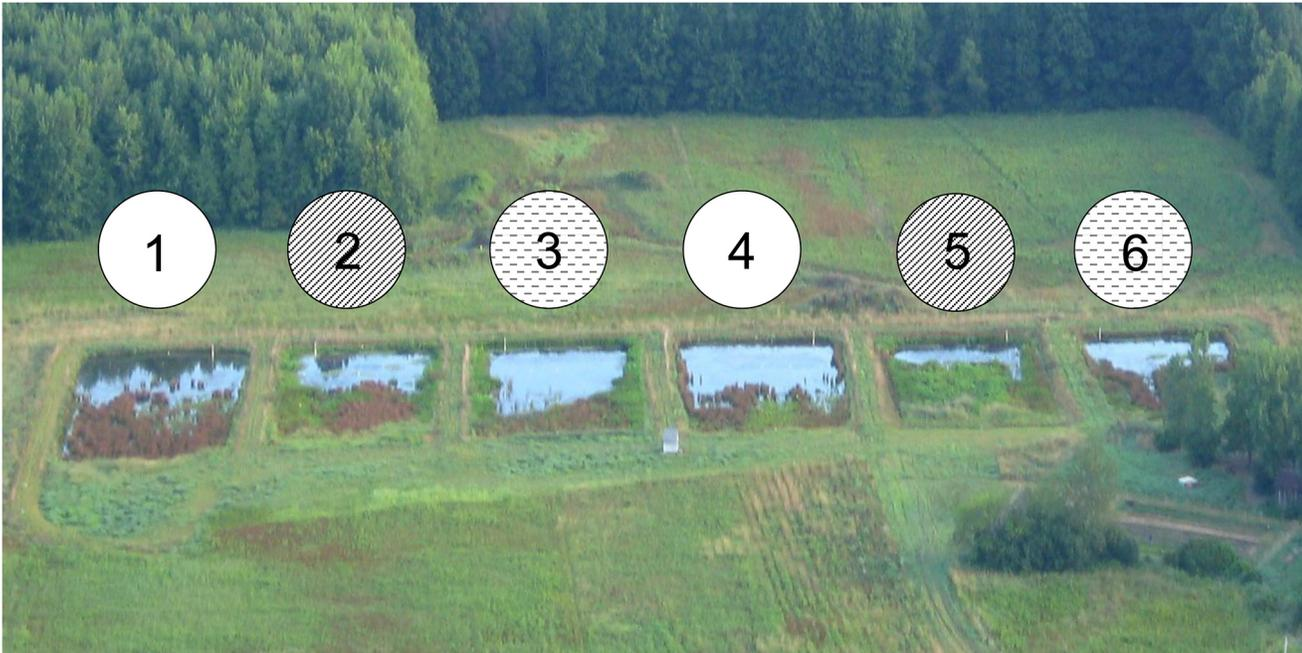
**Fig 1. Aerial view of experimental wetland cells taken in 2006.** “High-intensity” cells 2 and 5 were subjected to repeated plantings starting in 2003. “Low-intensity” cells 3 and 6 received initial planting and replanting the subsequent year. Cells 1 and 4 were unplanted. Cells 2, 3, and 4 were fertilized in 2010 and 2011.
