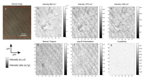
**Fig 2.** Raman images reproduce the alternation between the bright and dark incremental lines observed under microscopy a) optical image of the ROI showing alternating bright and dark lines of acellular cementum. b-d) spatial distribution of the intensity of Raman peaks  $960 \text{cm}^{-1}$ ,  $1070 \text{cm}^{-1}$  and  $1450 \text{cm}^{-1}$ ; e-g) spatial distribution of the physic-chemicals parameters Mineral/Organic, type-B Carbonatation and Crystallinity
