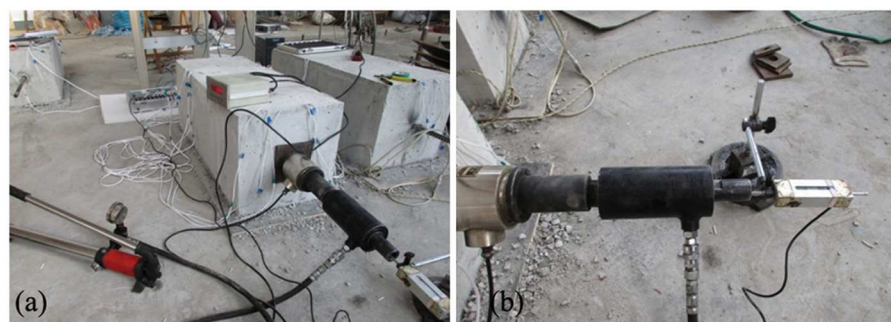
Fig 4. Loading setup for an anchor. (a) Physical model of an anchor pile. (b) Loading devices.
