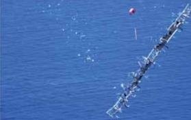
Helios Prototype breaks up in midair
