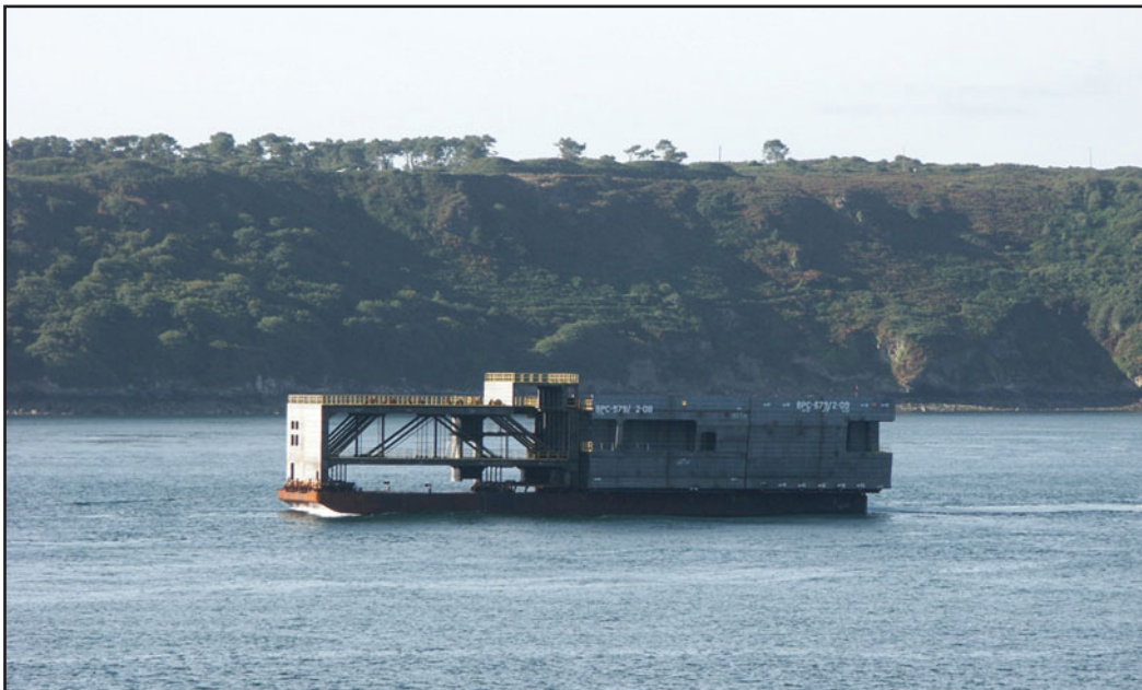
Figure G.3 Arrival in Brest of Blocks 2 and 3 Built in Poland on a Barge Towed by the Tug Atlant
