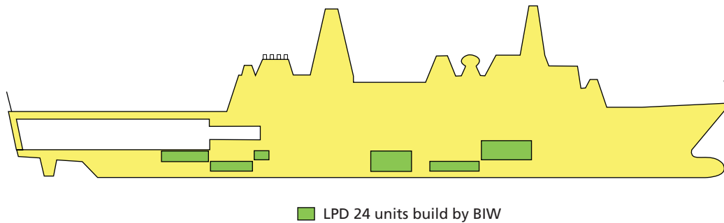
Figure C.1 LPD-24 Inboard Profile: Assembly Units
