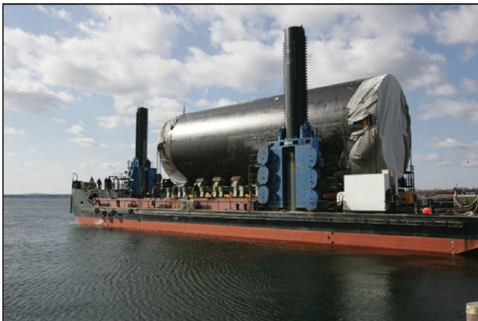
Figure D.2 A Supermodule Sits Aboard the Sea Shuttle at Quonset Point
