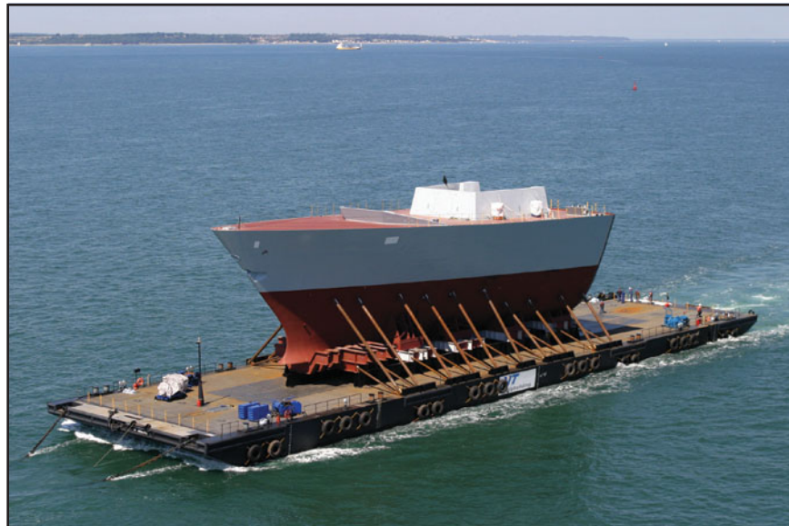
Figure E.4 Type 45 Bow Section on Barge Moving from Portsmouth to Glasgow
