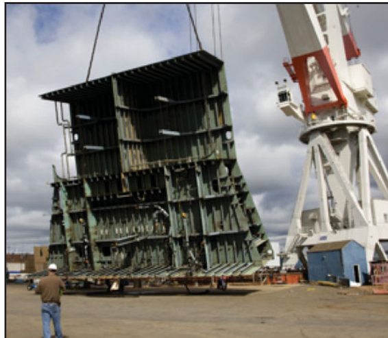
Figure C.2 Example LPD-24 Unit Being Lifted at Bath Iron Works
