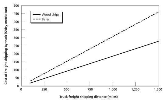
Figure 5.2 Impact of Trucking Shipping Distance on Truck Freight Costs for Wood Chips and Bales
