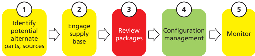
Figure 6.1 Basic Elements of Source Approval Request Processes for DoD and Commercial Airlines
