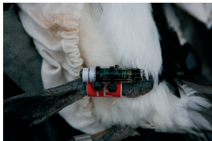
Figure 3. Above: Brünnich's guillemots ( Uria lomvia ) on a breeding ledge in the colony at Ossian Sarsfjellet, Kongsfjorden, Spitsbergen. Below: GLS (Geolocation Sensor) tag attached to a plastic ring on the leg of a Brünnich's guillemot. (Photos: Erlend Lorentzen, Norwegian Polar Institute)
