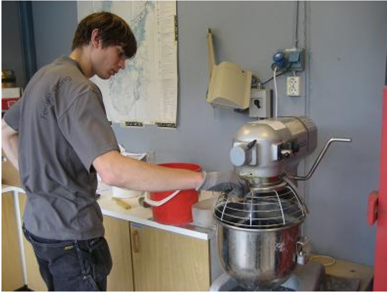
Figure 3 Mixing of mini concrete using a Hobart mixer.
