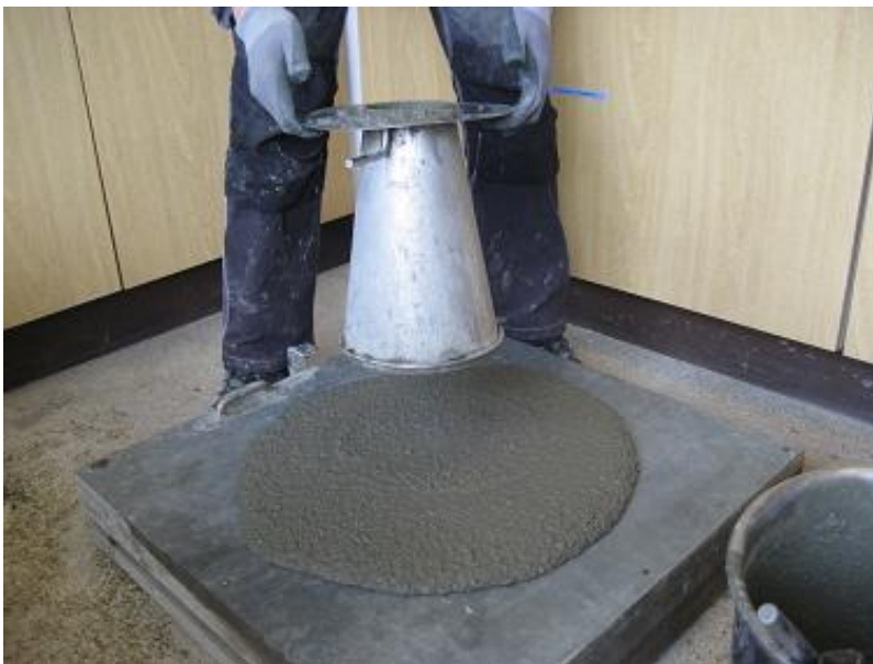
Figure 4 Ordinary slump cone and flow table. Measurement of slump and slump flow. Repeated measurements after 5 “dumps”.
