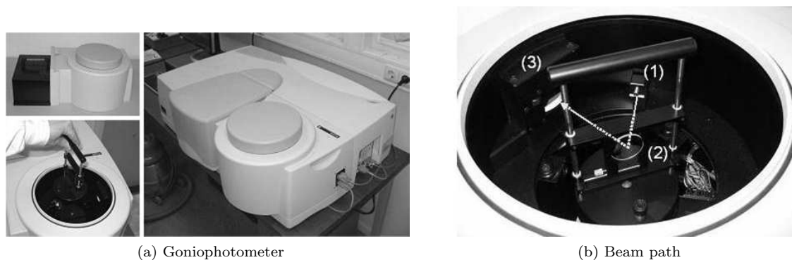
Figure 1: ARTA accessory installed in Perkin Elmer spectrophotometer 1a. The beam path in a reflectance measurement is shown in 1b. The sample (2) is illuminated by monochromatic light from the light periscope (1) and reflected into the integrating sphere detector (3). Reprinted by permission of OMT Solutions BV.
