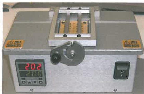
Figure A 2. DD6240 – Heated Adapter for Dage 4000 Plus shear tester.
