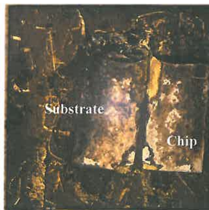
Figure 15. Micrograph of the fracture surface for a sample bonded with eutectic Au-Ge.
