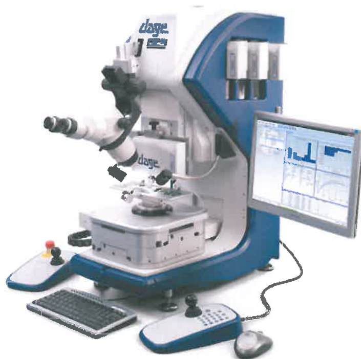
Figure A 1. Dage 4000 Plus shear tester.
