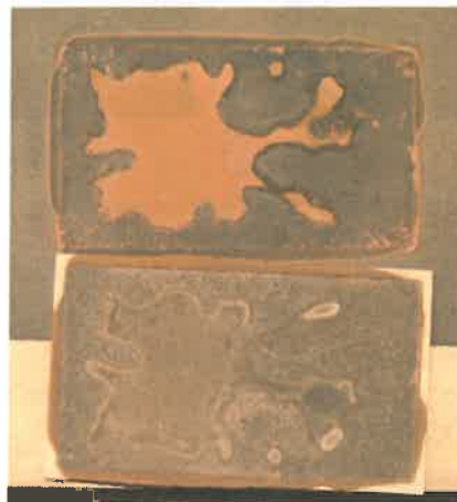
Figure 28. Image of the fracture surfaces of a Cu-plated \text{Si}_3\text{N}_4 substrate bonded to a Cu-plated AlSiC baseplate after thermal aging (2600 hours at 250 °C).
