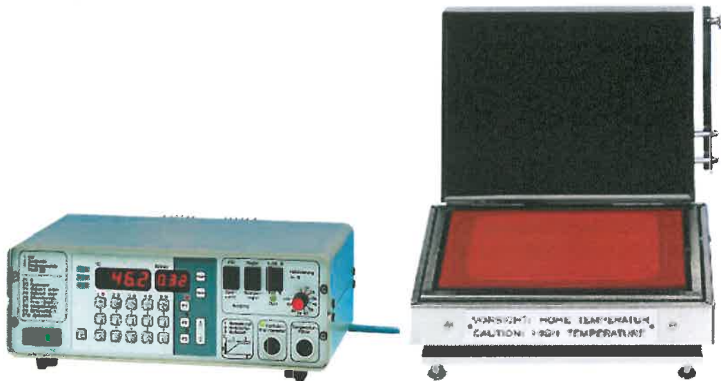
Figure A 3. Programmable controller (PR5-3T) and high temperature hot plate (PZ 28-3TD) bought from Harry Gestigkeit GmbH.
