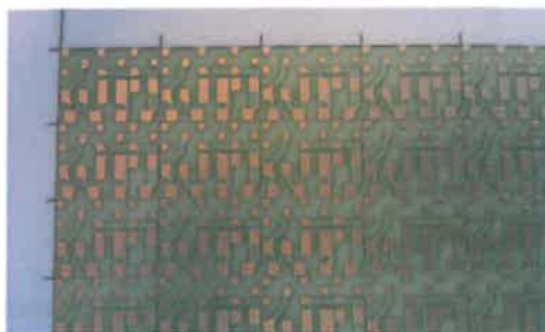
Figure 16. Test substrate for wire bond evaluation tests.
