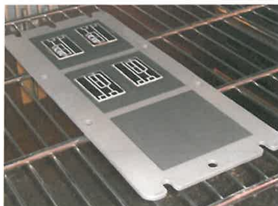
Figure 25. Si 3 N 4 substrates glued to an AlSiC baseplate with Duralco 4703. Two of the substrates contains three (six in total) Vishay PHT 2010 resistors glued with the same Duralco 4703.
