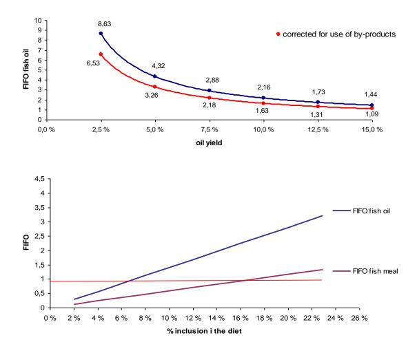
Figure 15FIFO as a function of the conversion efficiency of reduction fish into fish oil.b) FIFO ratio as a<br/>function of the inclusion level of fish meal and oil in the diet.Data from 2010 are used in the<br/>calculations (FCR = 1.3, inclusion level of fish oil was 16.6% of which 24 % came from trimmings<br/>and by products. The fish meal and oil yield from forage fish is 22.5 and 9.3 % respectively).
