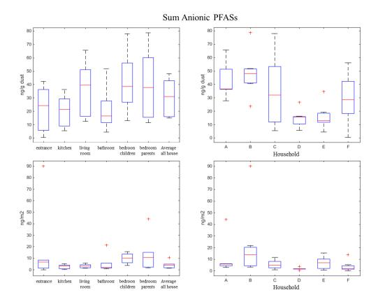
**Figure 4**. Boxplots of sum anionic PFASs in house dust in specific rooms (left) and individual households (right), in ng/g dust and  $ng/m^2$  respectively. Whiskers represent 5 and 95 percentiles, the boxes represents 25 and 75 percentile, and the red lines represent the median.
