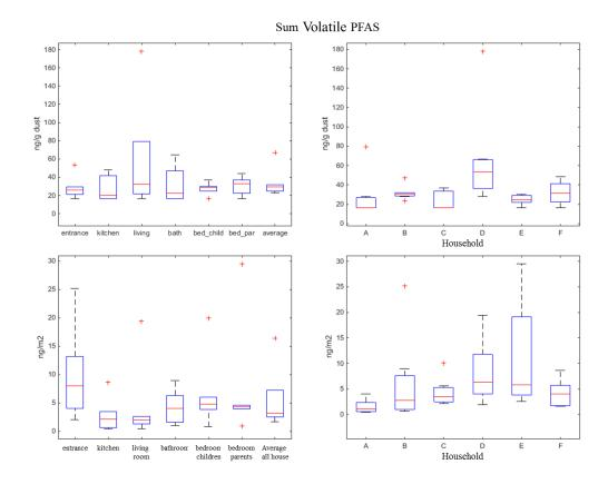
**Figure 5.** Boxplots of sum volatile PFASs in house dust in specific rooms (left) and individual households (right), in ng/g dust and  $ng/m^2$  respectively. Whiskers represent 5 and 95 percentiles, the boxes represents 25 and 75 percentile, and the red lines represent the median.
