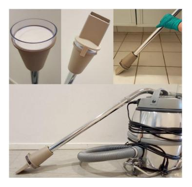
Figure 1. Sampling equipment for house dust in this study.
