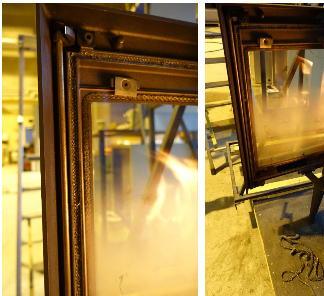
Figure 9: Woodstove door after removal of the gasket.
