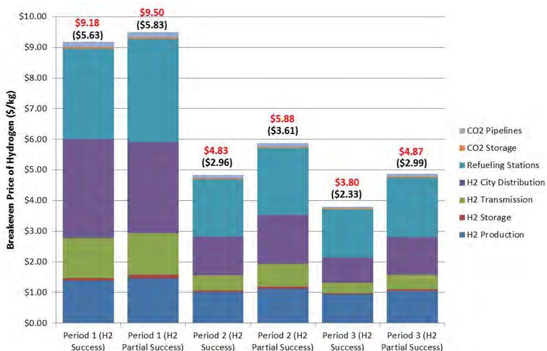
Figure 65: Breakeven price of hydrogen for three 10-year periods for the H 2 Success and H 2 Partial Success scenarios (price in parentheses is the equivalent price for a gallon of gasoline ($/gge) assuming that a HFCV has 63% better fuel economy than a gasoline HEV)
