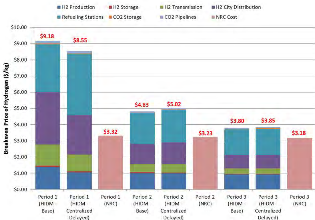
Figure 101: Breakeven price of hydrogen in each analysis period for the HIDM and NRC model (H 2 Success)
