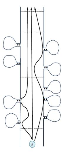
Figure 4.4. Schematic of an Acoustic-Tag, Release-Recapture Design to Estimate Juvenile Salmonid Survival, Site Use Patterns, and Near-Term Benefits of Site Use. Cross-river arrays (dotted line) and individual hydrophones (•) at estuary openings are delineated. Three possible fish tracks are illustrated.
