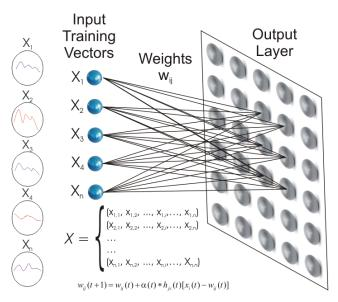
**Figure 3.3**. A Representation of the Single-Layer Self-Organizing Map (SOM) Process as it Presents Data to the Network, Competes, and Maps Organized Data Clusters to a Defined 1-D, 2-D, or 3-D Topology. The SOM provides the core signal classification engine within the ALCP.
