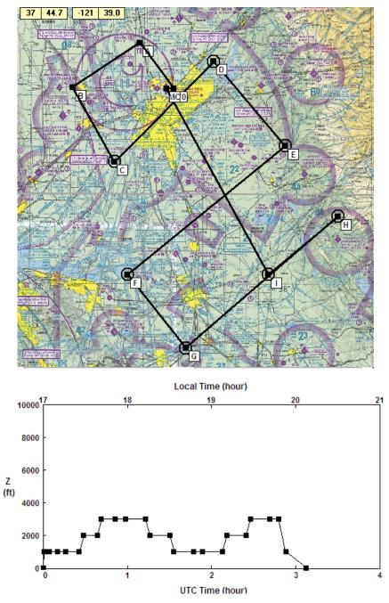
Figure 13. "Afternoon 2" Flight Plan.
