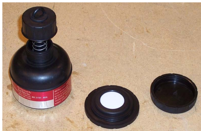
Figure 2. E-PERM® electret system (S-chamber, ST-electret, and storage cap).
