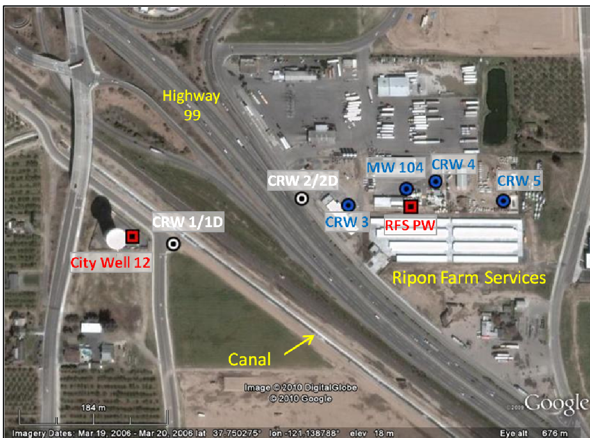
Figure 1. Wells sampled at Ripon, CA. Productions wells (Ripon City Well 12 labeled “Well 2” and Ripon Farm Services Production Well labeled “RFS PW”) are indicated by red squares; shallow monitor wells (CRW-3, CRW-4, CRW-5, and MW-104) are indicated by blue circles; and shallow and deep monitor well clusters (CRW-1 and -1D; CRW-2 and -2D) are shown as white circles. Screen intervals are listed in Table 1.
