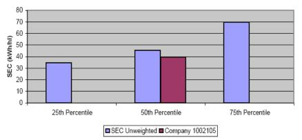
Figure 11 Benchmarking Electricity Use for Beer Production of a Company
