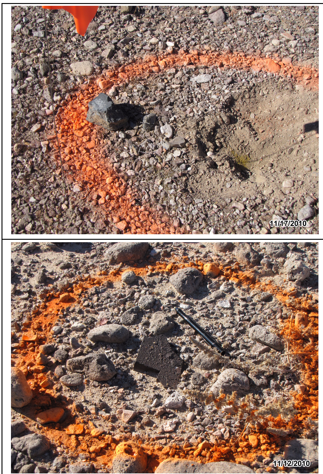
Figure D.1-1 Example of Oxidized DU (Top) and Example of DU-Contaminated Debris (Bottom)
