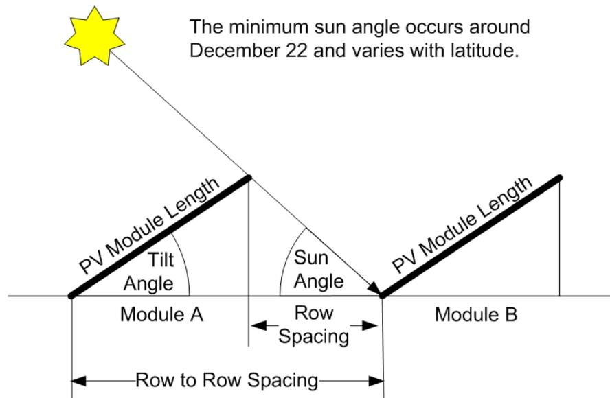
**Figure 4. Row spacing depends on the latitude and tilt of the PV modules**
