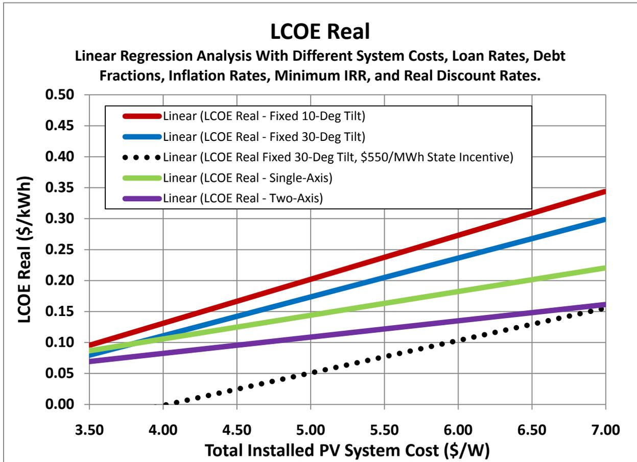
Figure 12. Linear regression analysis of statistical analysis of LCOE using ranges of values listed in Table 2 for four different types of PV mounting
