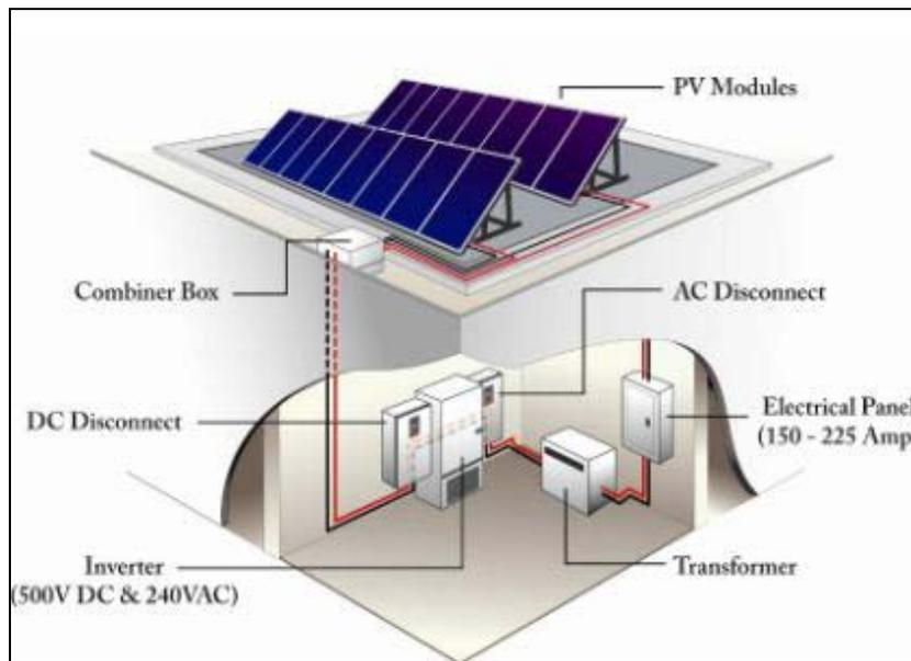
**Figure 1. Major components of grid-connected PV system**
