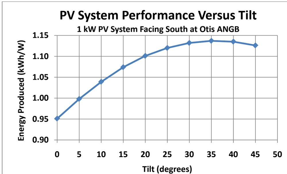
**Figure 2. Comparison of energy production for 1 kW PV system at Otis ANGB as a function of tilt**
