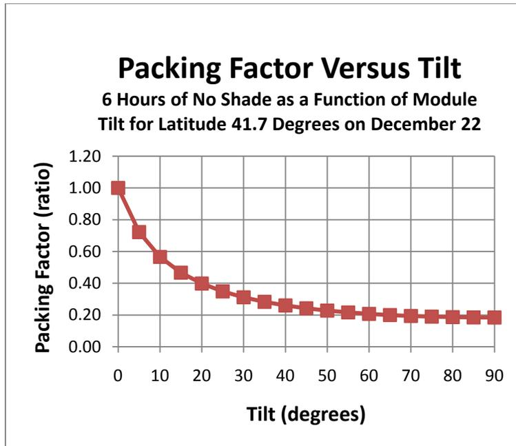
**Figure 5. Packing factor estimate versus tilt**
