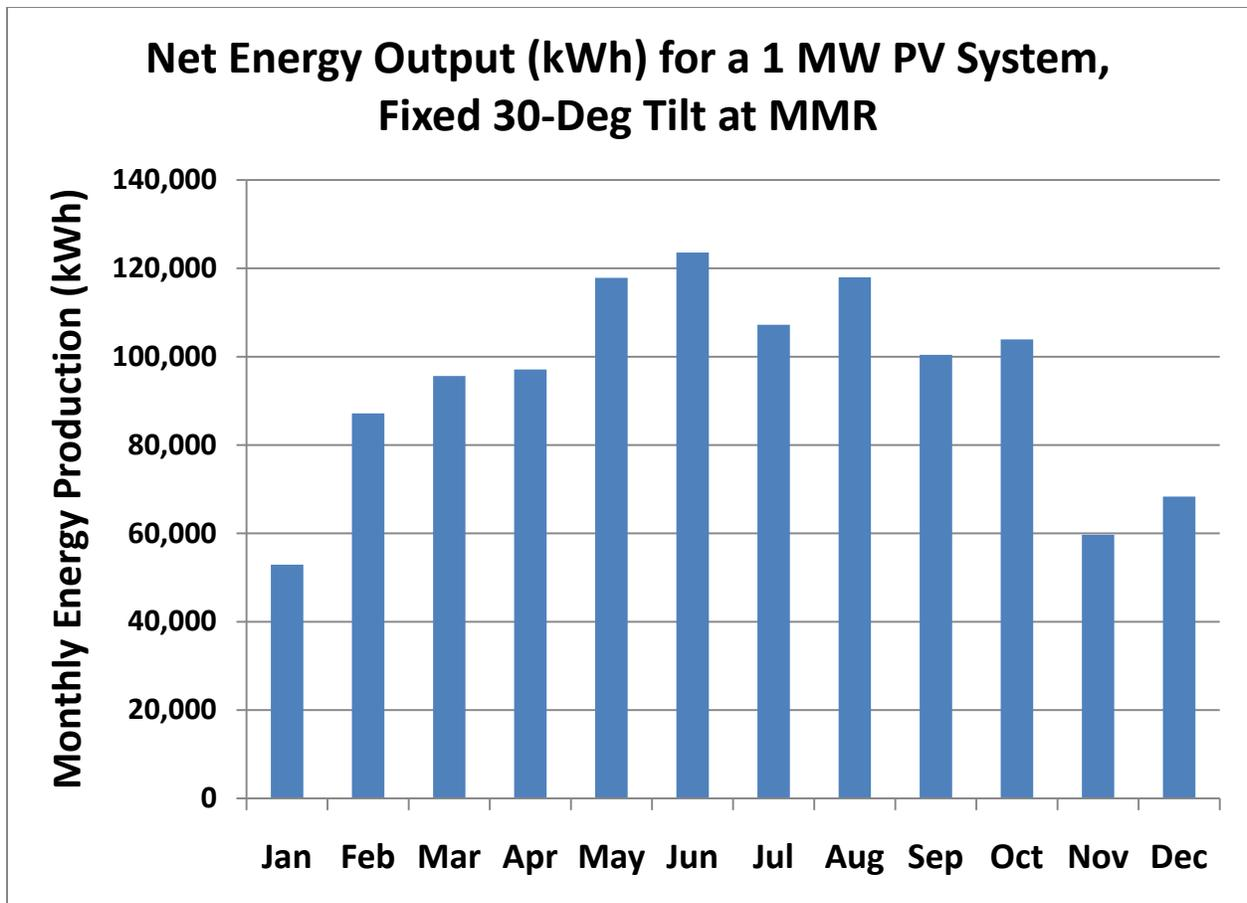
**Figure 3. Estimate of monthly energy production for a 1 MW PV system at MMR**
