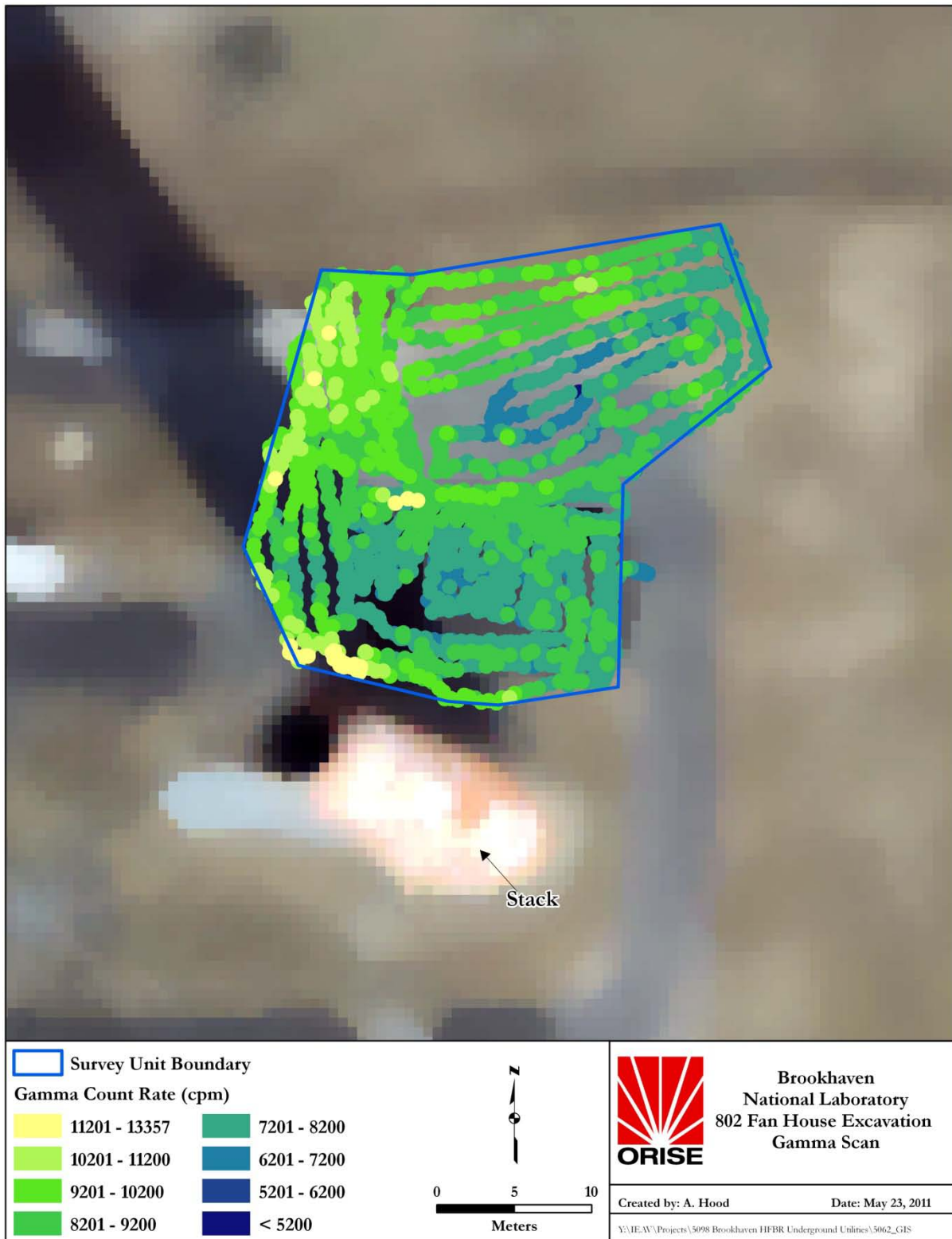
Figure A-3: Gamma Scans of the 802 Fan House Survey Area
