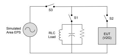
Figure 3. Unintentional islanding test circuit
