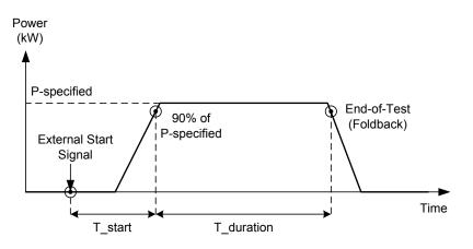
Figure 4. Power profile for a typical V2G converter during test with foldback
