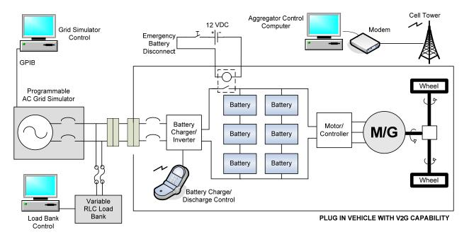
Figure 2. Example of V2G test setup
