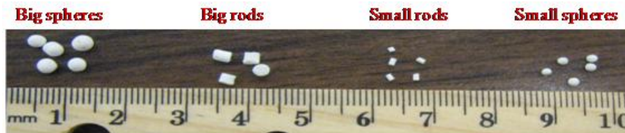
Figure 4-52 Comparison of size and shape of the pellets.
