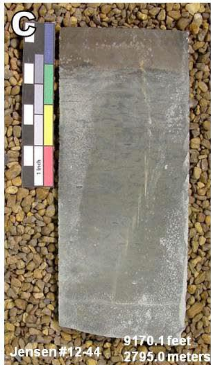
Figure 11. Core photos of facies F – bioturbated, shaly, dolomitic siltstone. This uppermost facies of the middle Bakken lies directly below the contact with the upper Bakken shale as seen in photos C and D.
