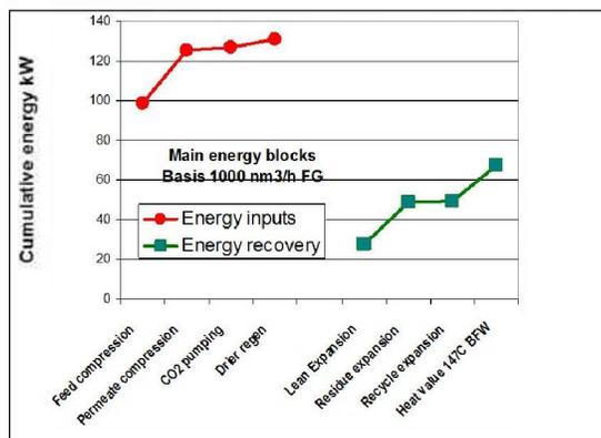
Figure 21. Simulation results showing cumulative energy demand (in red) and recovery (green) from the main energy intensive operations. Basis 1000 nm<sup>3</sup>/h flue gas. The gap between final red and green lines is the parasitic energy for CO<sub>2</sub> capture.
