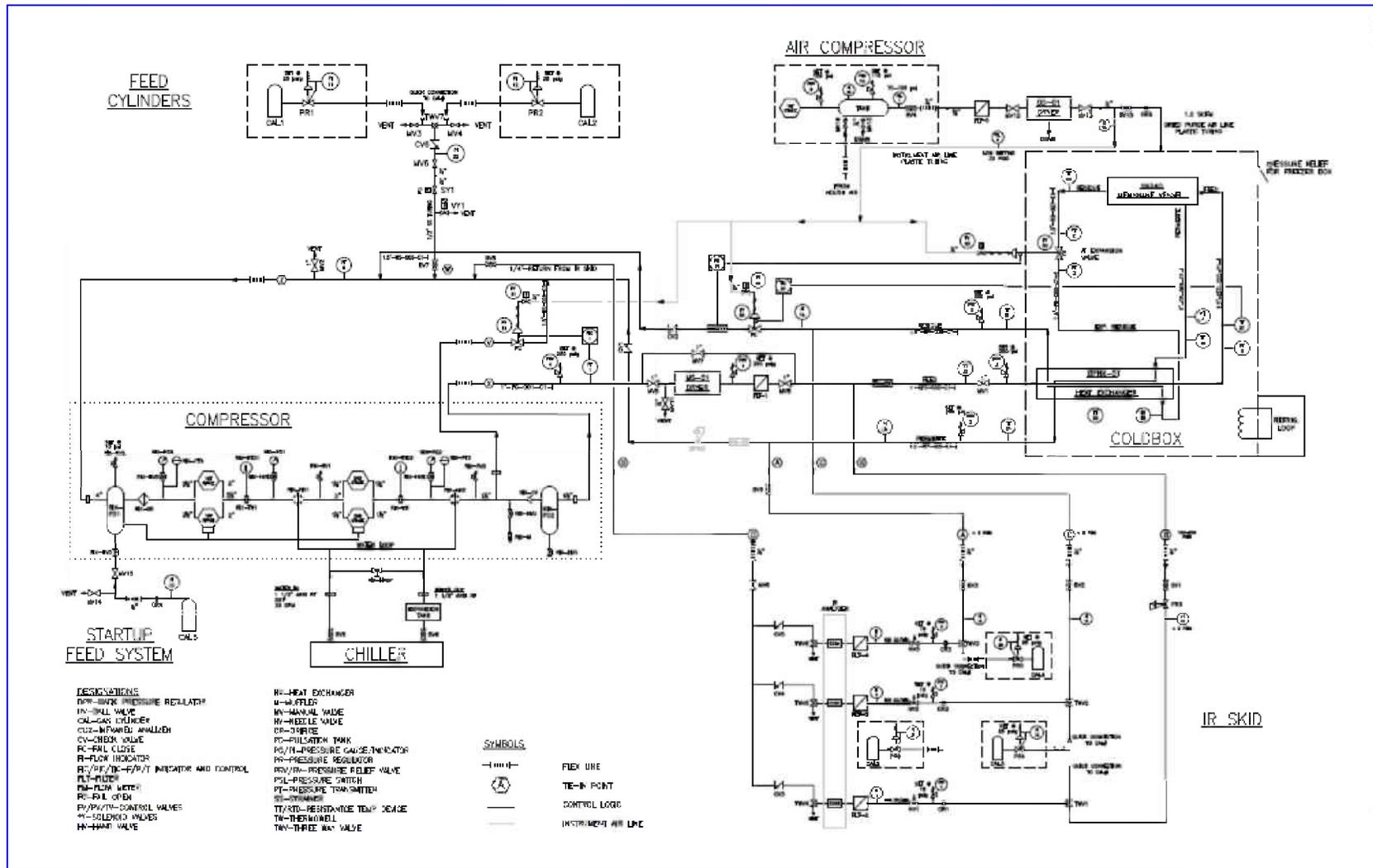
Figure 5. PID of integrated bench scale test skid
