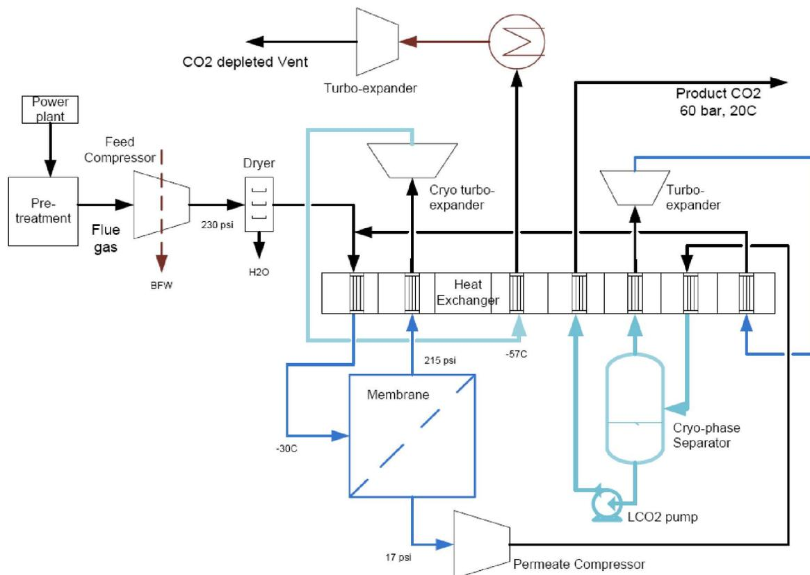
Figure 4: CO<sub>2</sub> Capture Process Schematic
