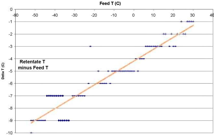
Figure 6. (6a) Feed gas temperature as a function of time on initial cool-own. (6b) Heat exchanger approach temperature as a function of feed gas temperature.
