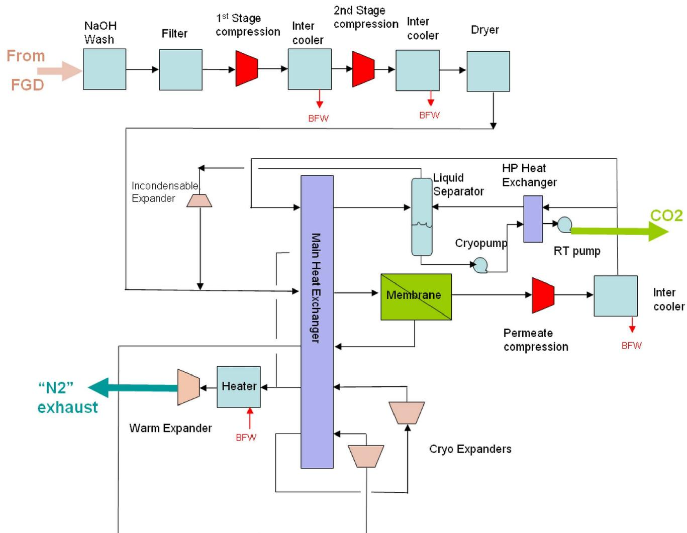
Figure 20: Block diagram showing equipment items in conceptual cold membrane process for CO<sub>2</sub> capture from FGD treated power point flue gas
