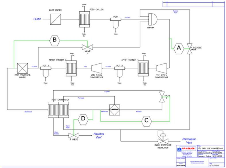
Figure 23. PFD of potential field test (0.1 MW scale) to demonstrate cold membrane operation with flue gas
