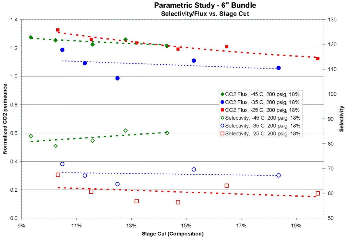
Figure 13: CO<sub>2</sub> Permeance and CO<sub>2</sub> / N<sub>2</sub> Selectivity as a Function of Stage Cut at Feed Temperatures of -45°, -35°, and -25°C at 200 psi Feed Pressure, and 18% CO<sub>2</sub> feed concentration
