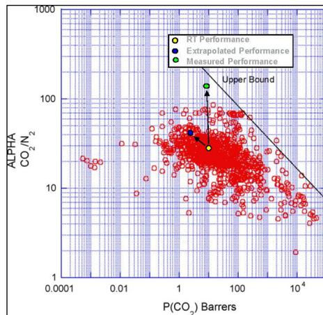
Figure 2. Plot of back-calculated equivalent permeability and selectivity at ambient temperature (yellow) and at -30°C (green) on a Robeson [11] plot for CO<sub>2</sub>/N<sub>2</sub>. The cold temperature estimate was made by estimating effective skin thickness of the hollow fiber from ambient temperature data for the fiber and dense film. The blue point shows the performance at -30°C predicted by extrapolation of data from 20-50°C while the green point is the actual performance at -30°C.
