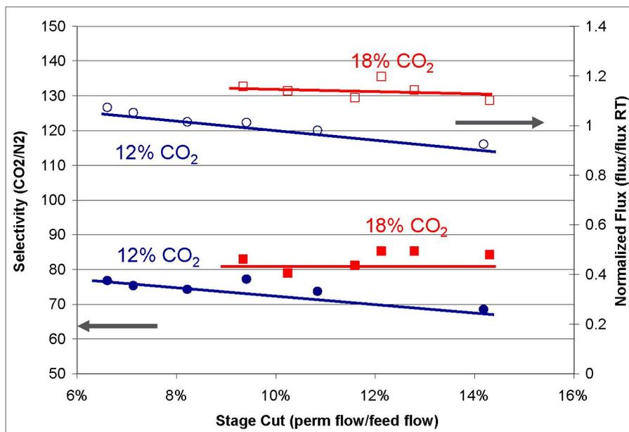
Figure 14: CO<sub>2</sub> Permeance and CO<sub>2</sub>/N<sub>2</sub> Selectivity as a function of feed CO<sub>2</sub> concentration (12% or 18%) as a function of stage cut; at -45°C / 200 psi. The right side Y-axis shows normalized permeance (CO<sub>2</sub> permeance at cold conditions / permeance at initial ambient temperature).
