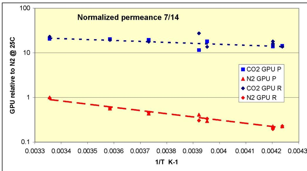
Figure 8. Normalized CO<sub>2</sub> and N<sub>2</sub> permeance at 200 psi, 18% CO<sub>2</sub>/N<sub>2</sub> as a function of feed temperature on 14-July-2011. The permeance values are calculated from either permeate (P) or residue (R) compositions and then normalized as per initial ambient temperature N<sub>2</sub> permeance.
