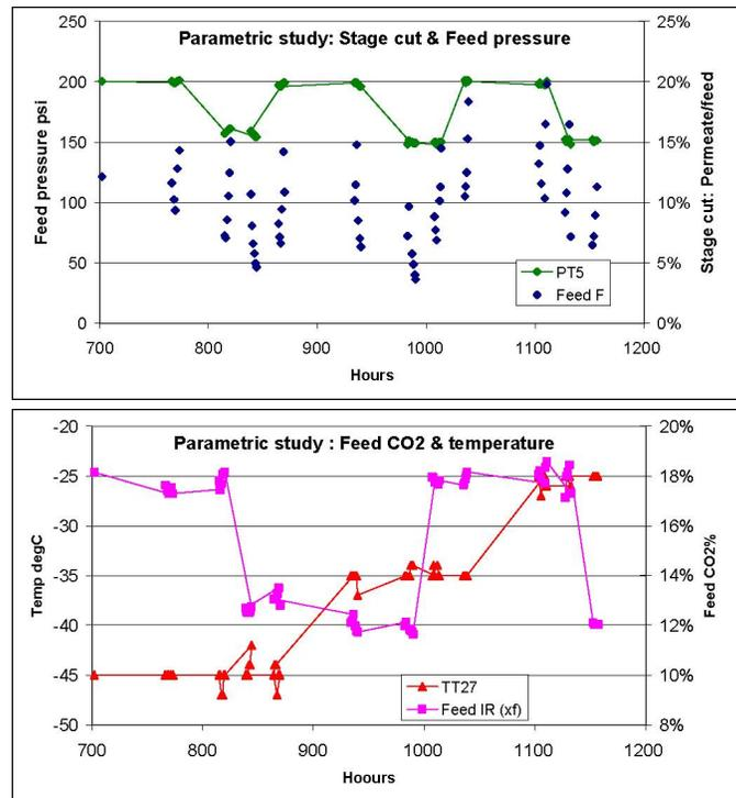
Figure 11: Parametric Variation for Performance Map with 6" Bundle Testing
