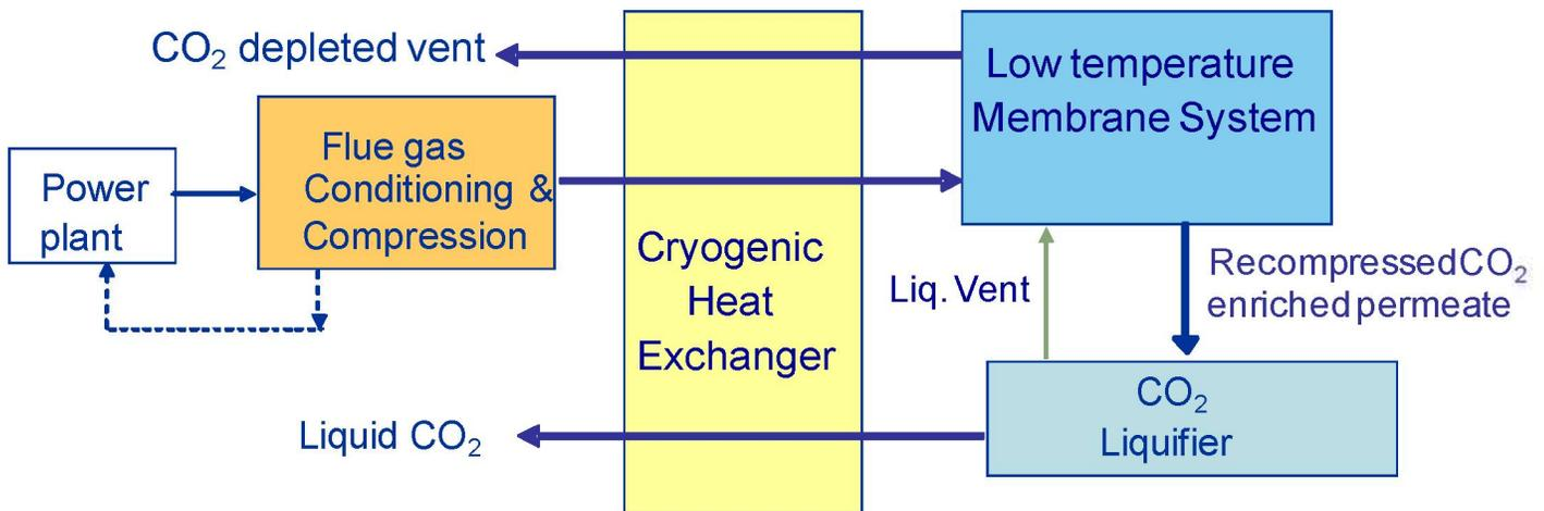
Figure 1. Sub-Ambient Membrane System for CO<sub>2</sub> separation
