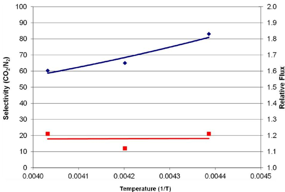
Figure 15 : Final parametric study: temperature dependence of membrane permeance-selectivity at 200 psi, 18% feed CO<sub>2</sub>. The right side Y-axis shows normalized permeance (CO<sub>2</sub> permeance at cold conditions / permeance at initial ambient temperature).
