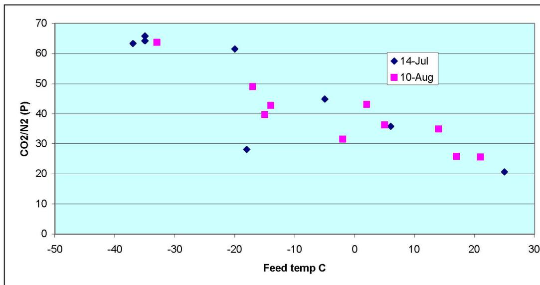
Figure 10.  $CO_2/N_2$  selectivity at 200 psi, 18%  $CO_2/N_2$  as a function of feed temperature; comparison of data taken on 14-July -2011 and 10-August-2011.
