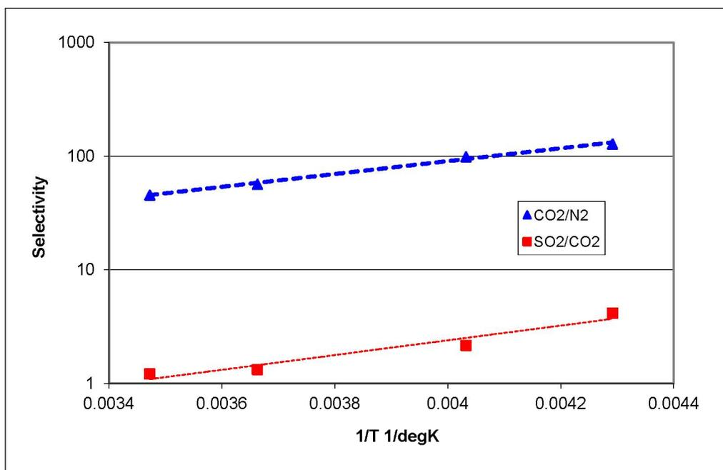
Figure 18: Temperature dependence of CO<sub>2</sub>/N<sub>2</sub> and CO<sub>2</sub>/SO<sub>2</sub> Selectivity for Laboratory Permeator. 100 ppm SO<sub>2</sub>, 20% CO<sub>2</sub> in N<sub>2</sub> at 140 psi
