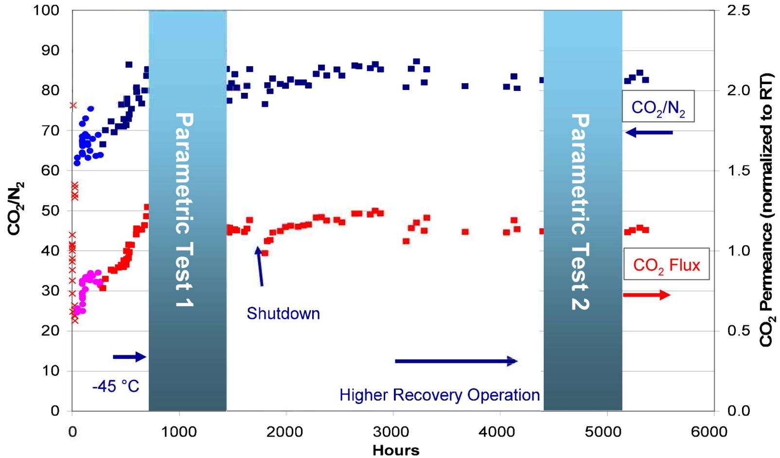
Figure 17:  $CO_2$  Permeance and  $CO_2/N_2$  Selectivity for 6" Bundle Testing. Normal test conditions: -45C, 200 psig, 18%  $CO_2$  in feed. The right side Y-axis shows normalized permeance ( $CO_2$  permeance at cold conditions /permeance at initial ambient temperature). The bundle was operated with an average  $CO_2$  recovery of ~ 80% after 3000 hours and ~ 50% at previous times.
