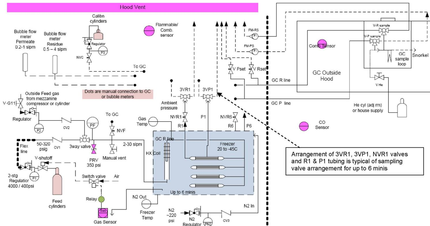
Figure 7. Schematic of cold membrane test system for feed gases with toxic components (SO<sub>2</sub>, NO)
