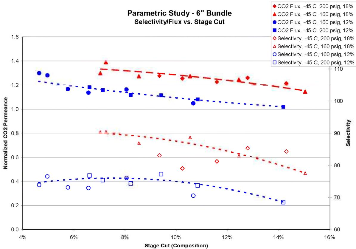
Figure 12: CO<sub>2</sub> Permeance and CO<sub>2</sub> / N<sub>2</sub> Selectivity as a Function of Stage Cut at Feed Temperature of -45°C, Feed Pressures of 200 and 160 psi, and Feed CO<sub>2</sub> Concentrations of 18% and 12%
