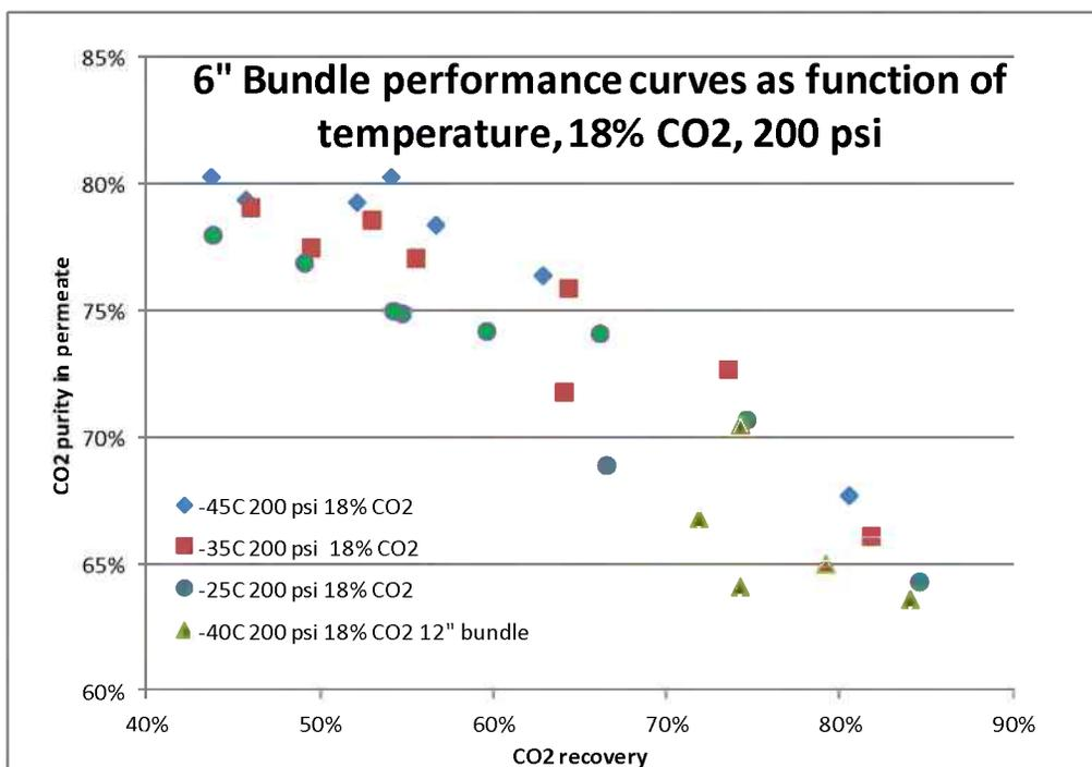
Figure 16 : Temperature dependence of 6" bundle membrane performance shown as plots of % CO<sub>2</sub> in permeate as a function of CO<sub>2</sub> recovery in the membrane at 200 psi, 18% feed CO<sub>2</sub>. Data curves are at -25°, -35° and -45°C. This plot also includes data for the 12" bundle at -40 °C, 200 psi, 18% feed CO<sub>2</sub>.
