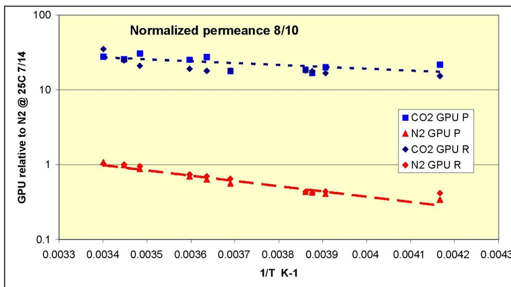
Figure 9. Normalized CO<sub>2</sub> and N<sub>2</sub> permeance at 200 psi, 18% CO<sub>2</sub>/N<sub>2</sub> as a function of feed temperature on 10-August-2011. The permeance values are calculated from either permeate (P) or residue (R) compositions and then normalized as per initial ambient temperature N<sub>2</sub> permeance on 14-July-2011.
