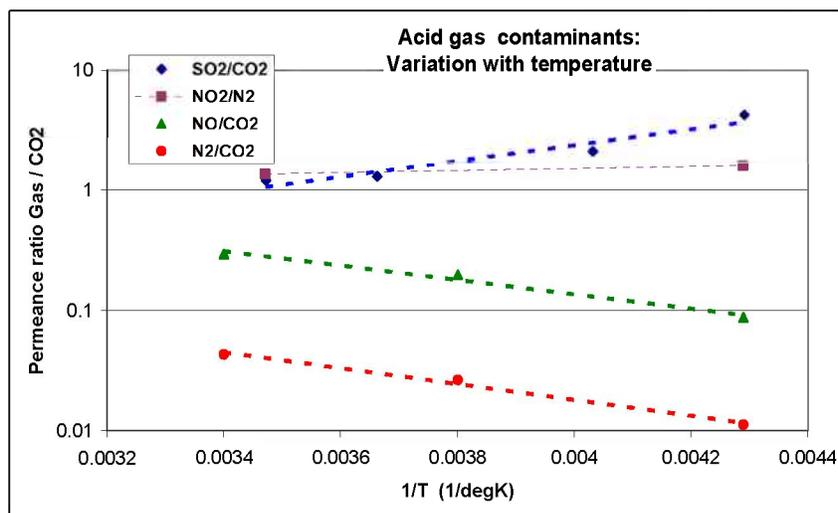
Figure 19: Temperature dependence permeance ratio (Gas permeance / CO<sub>2</sub> for SO<sub>2</sub>, NO<sub>2</sub>, NO, and N<sub>2</sub>. Data based on laboratory mini-permeator studies with 20% CO<sub>2</sub> in N<sub>2</sub> at ~ 140 psia containing 100 ppm of each acid gas
