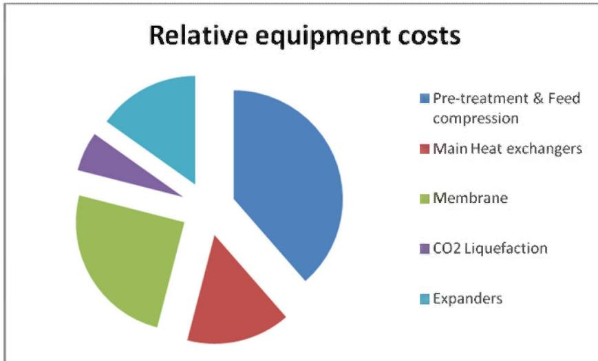
Figure 22. Relative capital cost (non-installed) for major equipment blocks of conceptual hybrid cryogenic + cold membrane process for 90% CO<sub>2</sub> recovery from a 550 MW (net) coal power plant.
