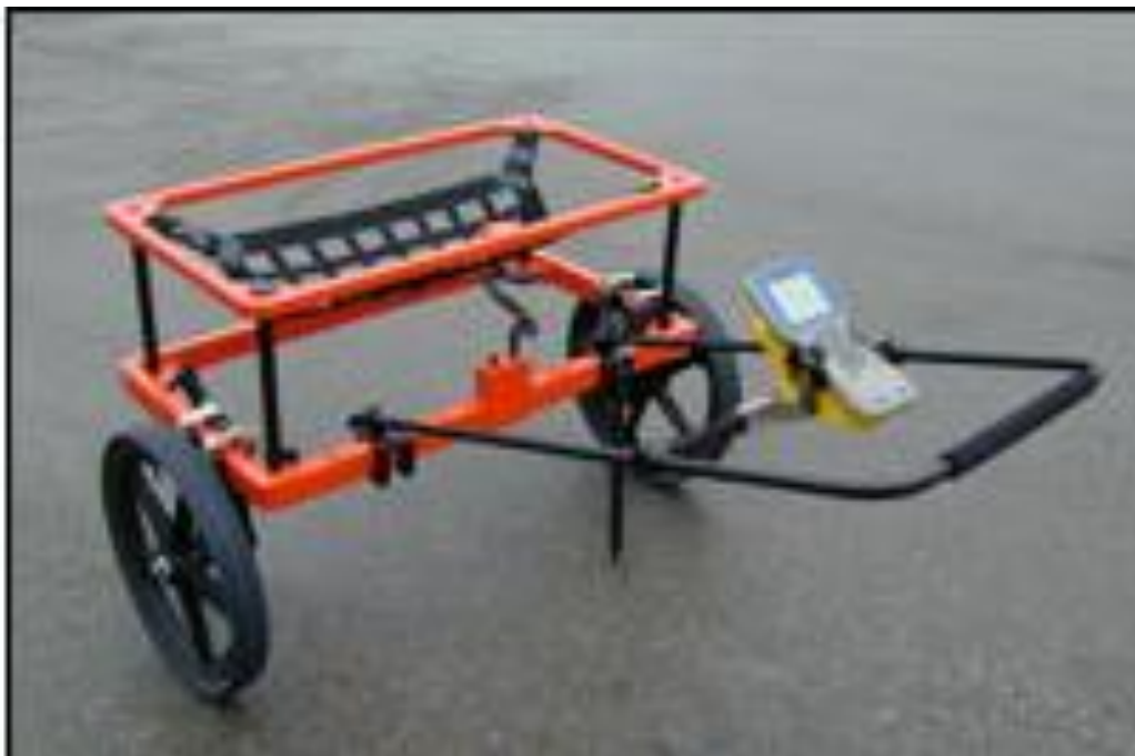
Figure 1 Photo of the EM61-MK2 with Wheels Supporting Coils (Geonics, 2011)
