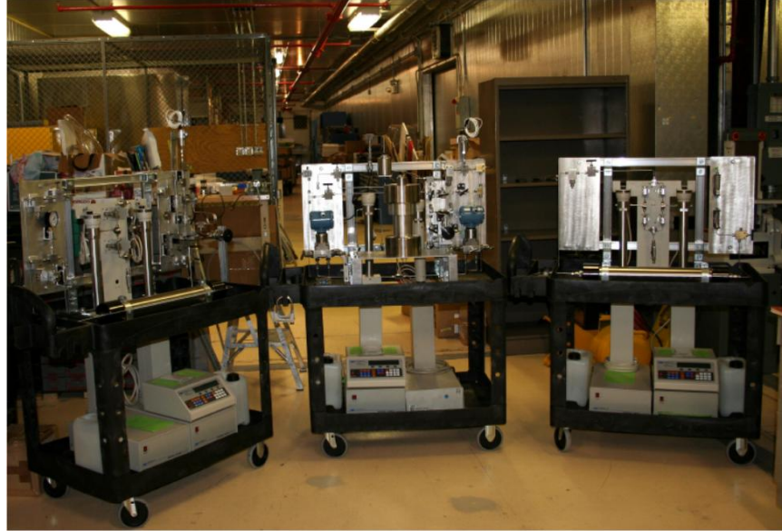
Figure 1. Overview of triaxial coreflood system. The system is portable to allow experiments at tomography facilities and is constructed on three separate, mobile carts. The middle cart contains the triaxial coreholder, pumps for confining pressure and axial load, pressure transducers, and fluid sampling. The right cart contains the brine delivery system, which includes two pumps and an accumulator for delivering continuous brine flow. The left cart contains the CO 2 delivery system, which includes two pumps, an accumulator, and a fluid sampling port. On all three carts, the pumps are located on the lower shelf.
