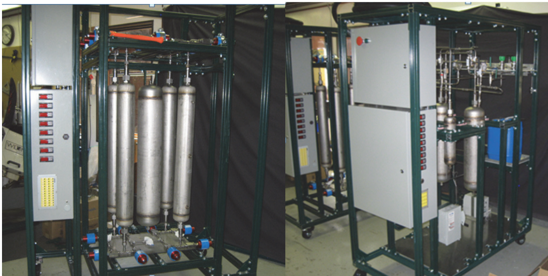
Figure 70. CO 2 Adsorption Unit (Left) Gas Conditioning Unit (Right) before installing inside the NEMA Enclosures.
