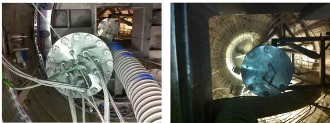
Figure 4-4. PRACLAY In Situ Experiment at HADES URL: Photo on left shows hydraulic seal from the outside, with an access hole to the right which soon will be closed. Photo on right was taken from access hole into the heater gallery section, which is currently being backfilled.
