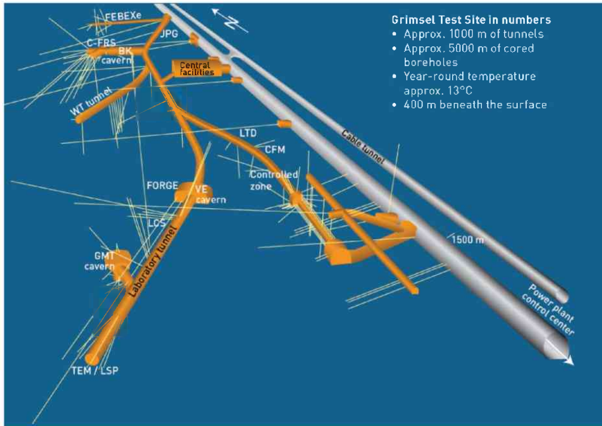
Figure 4-6. 3D view of layout of the Grimsel Test Site in Switzerland (NAGRA, 2010).
