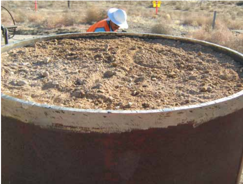
Photograph 17: CAS 03-99-19 (TEJON), Soil in Casing Over the Sampling Can at TEJON, 11/08/2011
