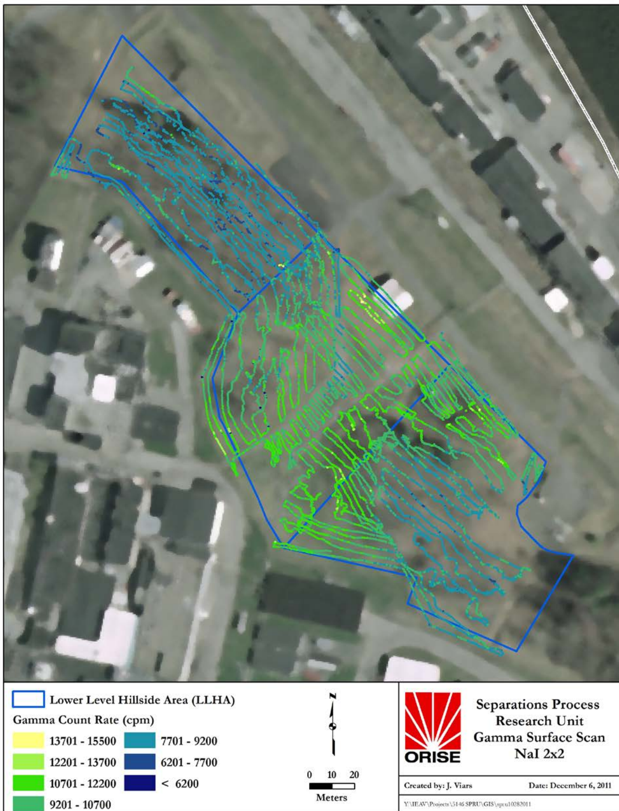
Figure A-3. SPRU Lower Level Hillside Area Gamma Surface Scans with 2x2 Detector
