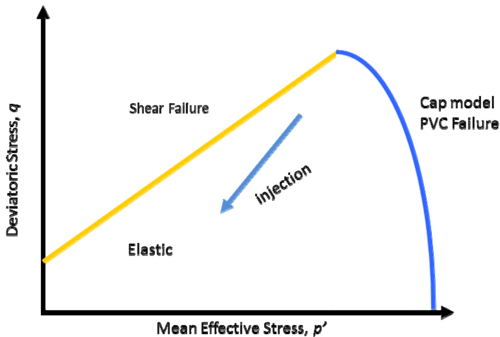
Figure 9. Injection reservoir stress path in q - p' space with higher slope than the failure line
