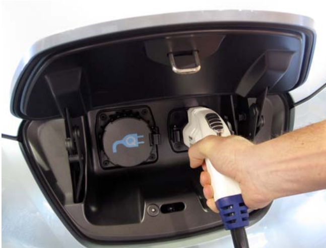
Figure 5. The standard EVSE connector fits into the standard receptacle. Photo by Andrew Hudgins, NREL/PIX 17634
