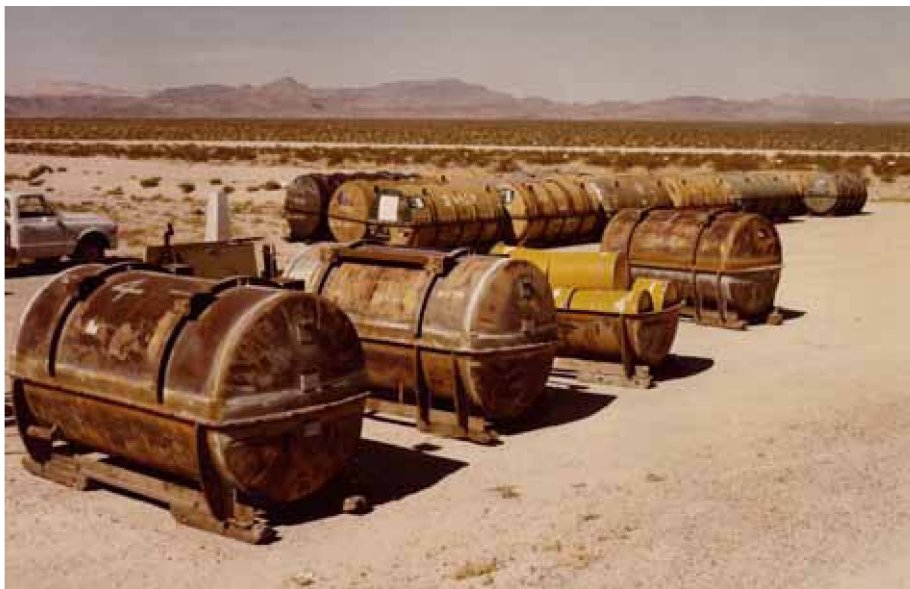
FIGURE A-1. STEEL DRUMS OVER-PACKED INTO LARGER STEEL CONTAINERS AT THE AREA 5 RADIOACTIVE WASTE MANAGEMENT SITE
