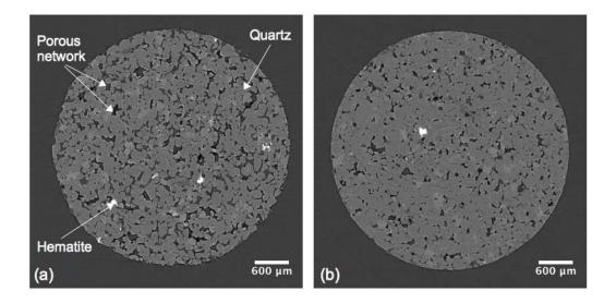
Figure 1. Sample horizontal CT slices from Aztec sandstone. (a) Outside compaction band and (b) inside compaction band.
